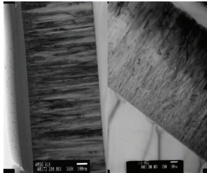
Fig. 3. TEM micrographs of high (left) and low (right) quality AlN films.
